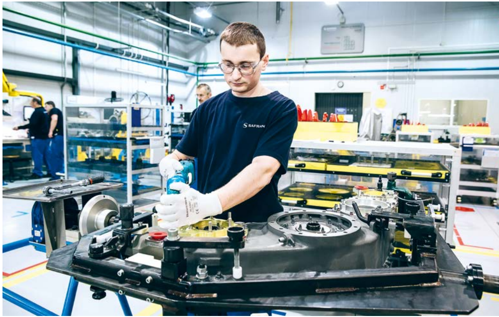
Mateusz Fitol , Safran Transmission Systems Poland employee, assembling a LEAP power transmission, also called an accessory gearbox.
