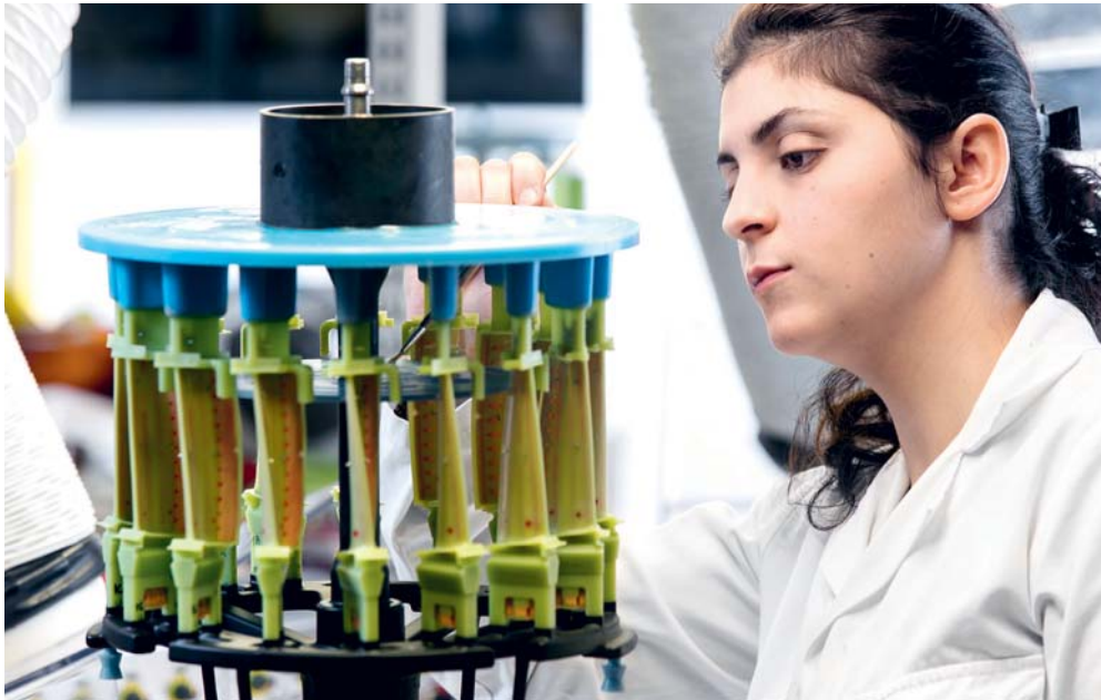
Preparing wax models at the Gennevilliers foundry.
