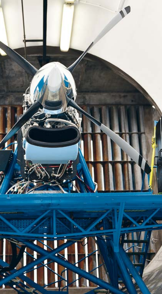
Tech TP ready for testing on a test cell dedicated to turboprop engines at the Tarnos plant in southwest France.
