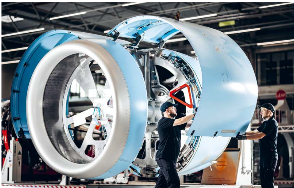
Integrating the nacelle on a LEAP-1A engine for the A320neo at the Safran Nacelles facility in Hamburg.
