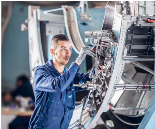
Top: the Ariane 6 launcher. Bottom: mobile assembly line for A320neo nacelles at the Safran Nacelles plant in Le Havre.
