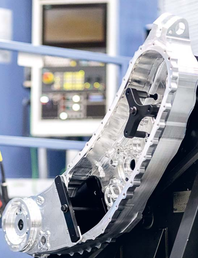
Power transmission case for the LEAP-1B , produced at our new five-axis machining center.
