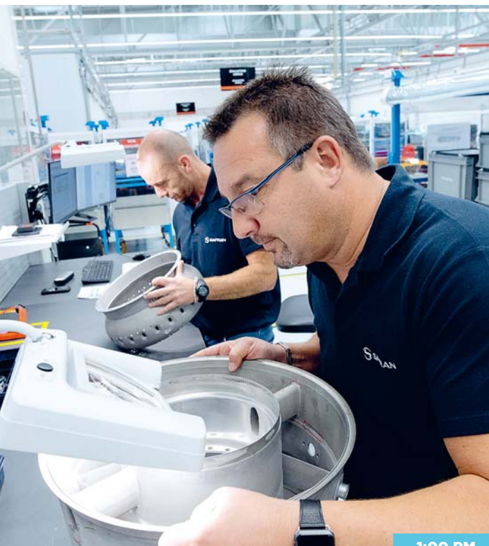
Employees can use another technique —visual inspection!— to identify the extent of damage to parts.
