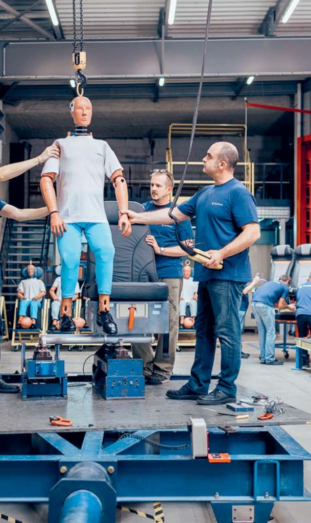
Left: Safran Seats Issoudun teams strap a dummy into a seat for a crash test.
