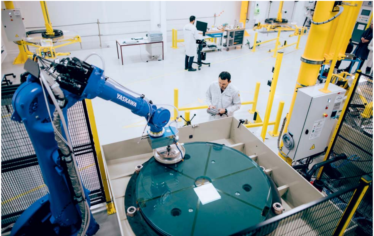
Start of a polishing operation by robotized machinery to ensure surface quality to within a nanometer.
